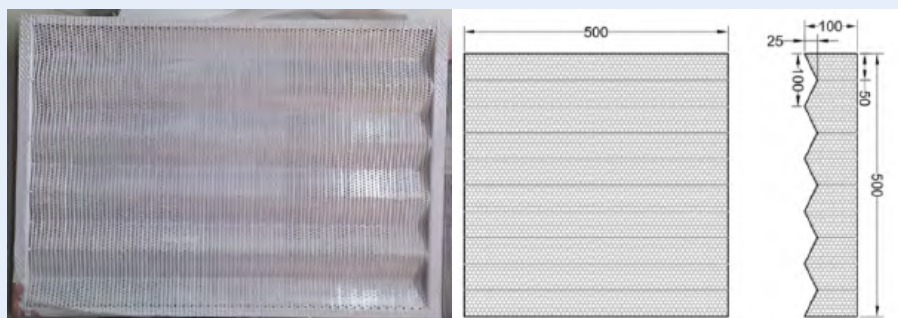
Composite panels fabricated for frequency specific sound absorption, ready for laboratory and field testing.
